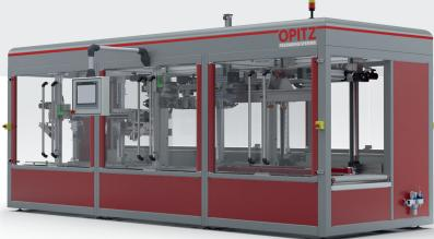
Sustainable and resource-saving packaging process with fully automatic height detection, minimization of package height, and secure sealing. There are two sealing methods:
